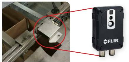
The AX8 camera is set up to look at predefined areas of the flaps where glue should be applied, and verify spot sizes and their temperatures.
